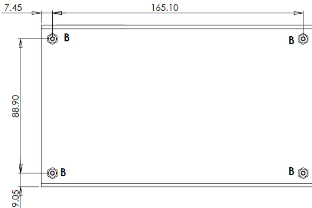
**B** 4 OFF FIXING HOLES FOR M3
