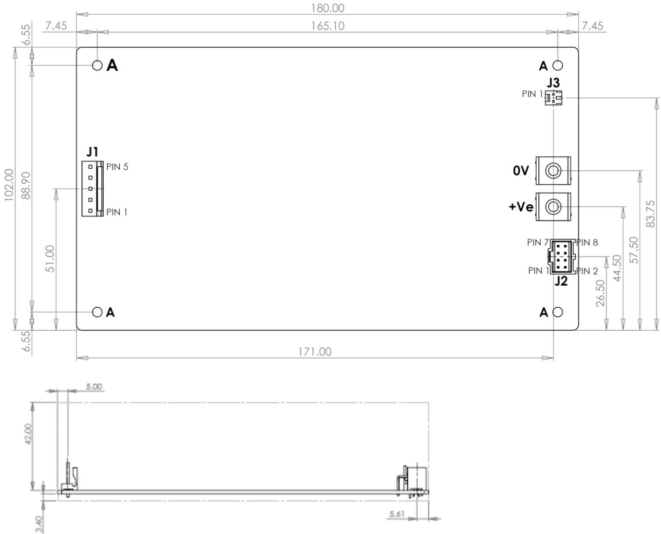
**A** 4 OFF HOLES Ø 3.5mm CLEARANCE FOR M3 FIXINGS.
