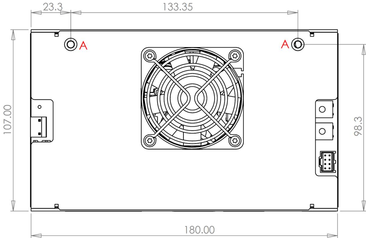
A 2 OFF FIXING HOLES FOR M3
