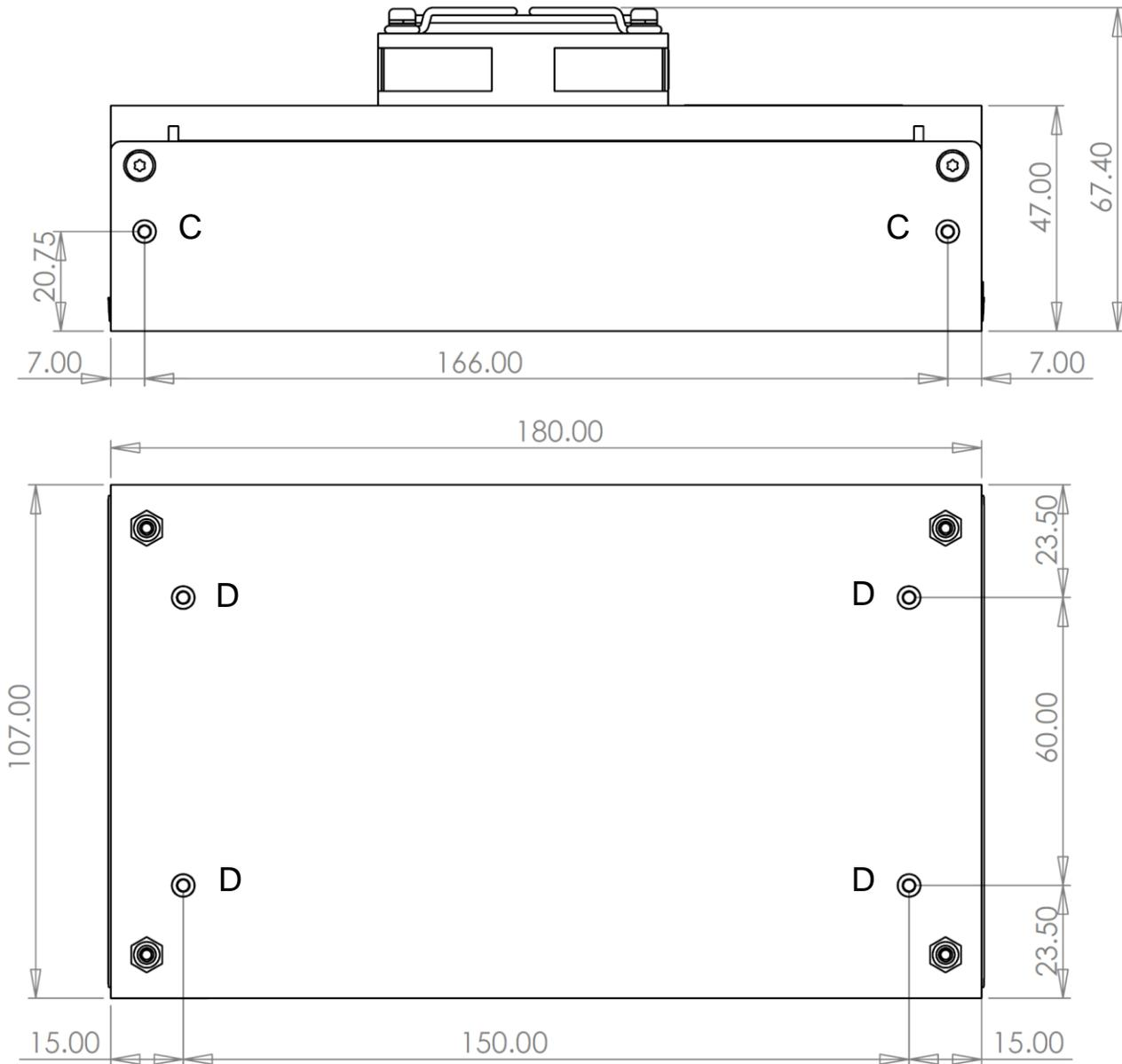
C 2 OFF FIXING HOLES FOR M3 MAXIMUM PENETRATION OF 3MM
