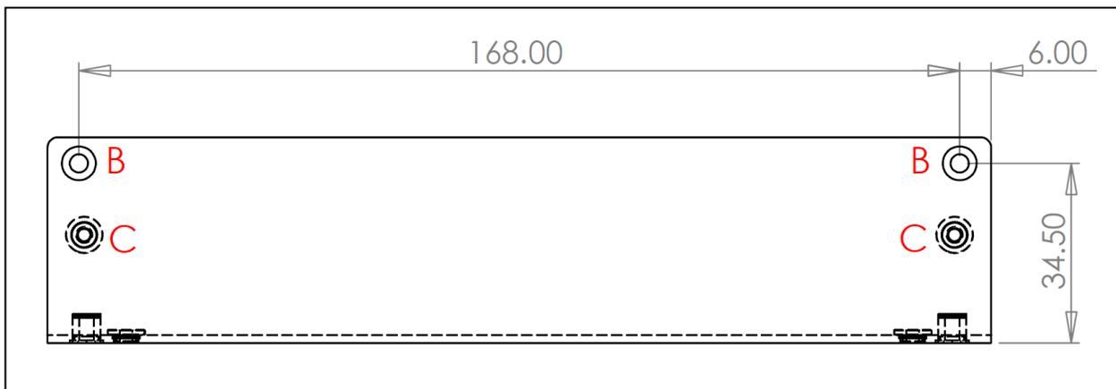
C 2 OFF FIXING HOLES FOR M3 MAXIMUM PENETRATION OF 3MM
