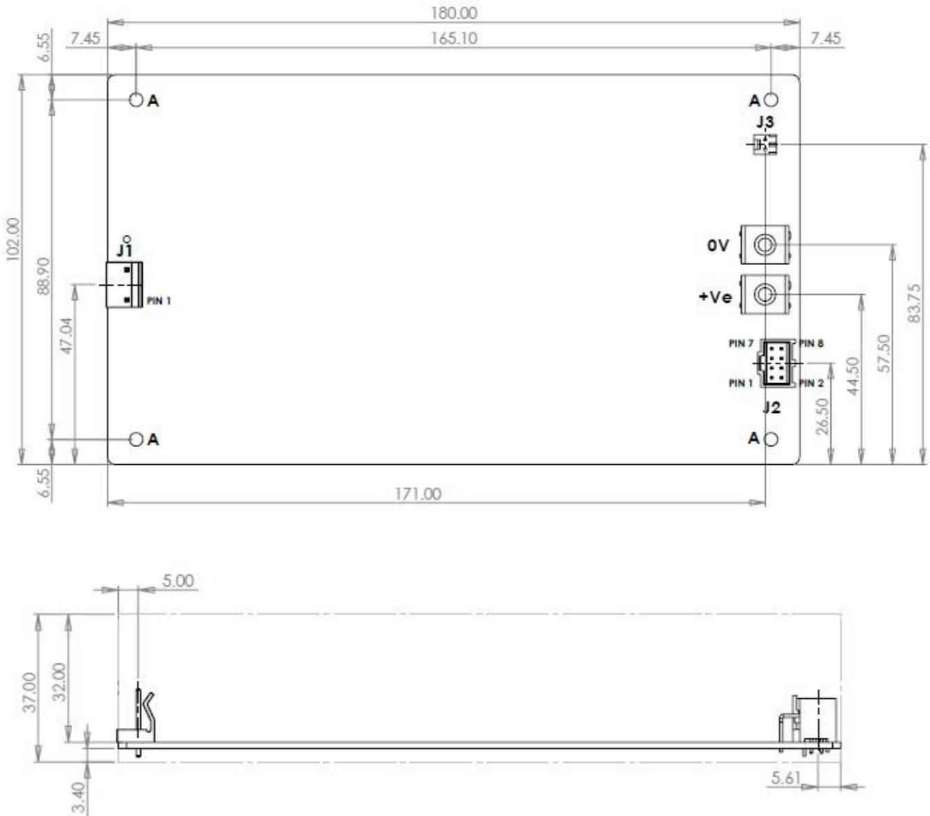
A 4 OFF HOLES Ø 3.5mm CLEARANCE FOR M3 FIXINGS.
